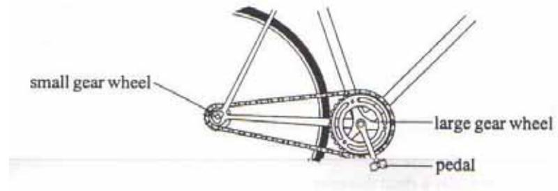
When you pedal two full cycles, how many times will the back wheel turn?
