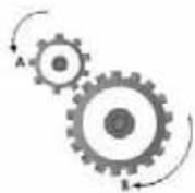
The figure above shows two gears labeled A and B. When you count the number of teeth of gear A you will get 9 teeth. Gear B has 18 teeth. When gear A rotates once then gear B has passed only half way. Why? The solution lies in:
